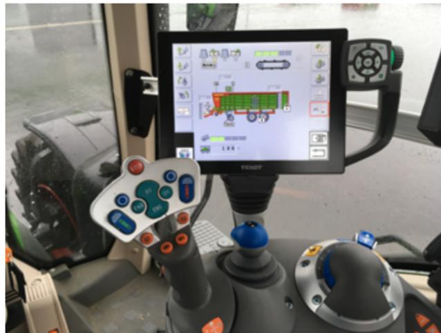
Due to the compatibility of the Strautmann ISOBUS control (ISOBUS AEF certification), most varied terminals can be used for the Strautmann forage wagons. Thus, depending on the tractor type, all machine functions can also be operated via the tractor joystick.
