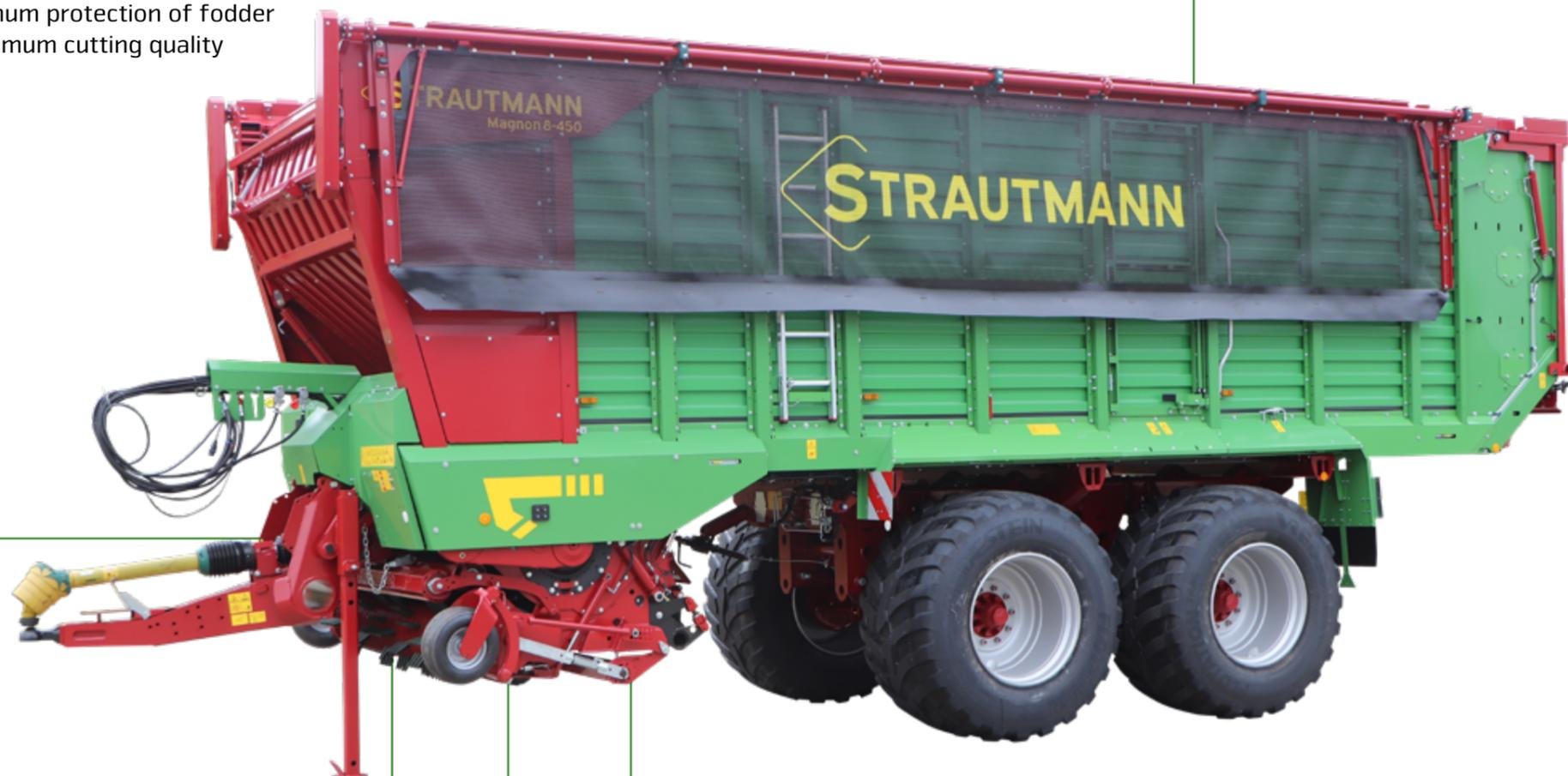
**Minimum wear** and optimum adaptation to the ground due to the innovative Flex-Load pick-up with plastic tines
