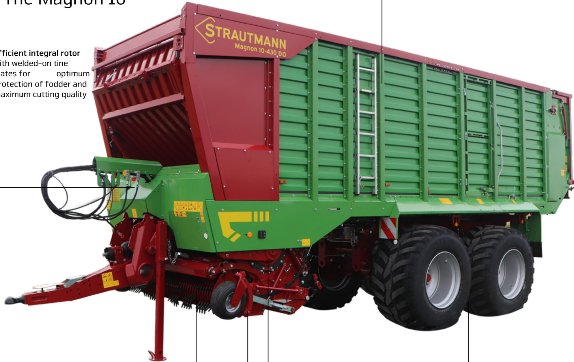
Minimum wear and optimum adaptation to ground due to the innovative Flex-Load pick-up with plastic tines
