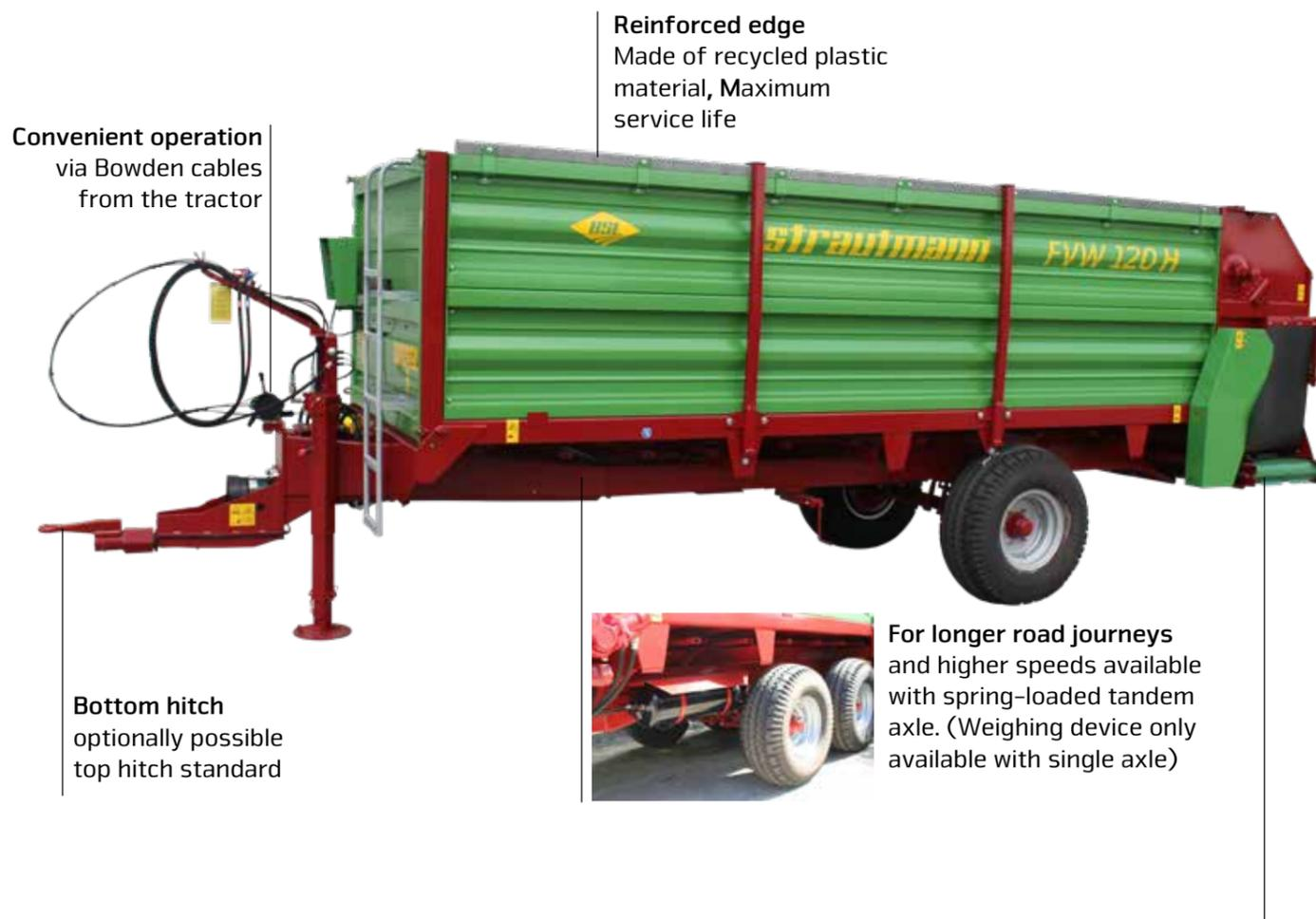
Convenient operation via Bowden cables from the tractor
