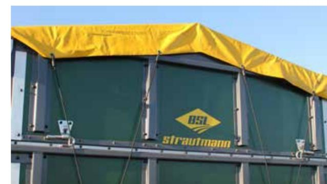
The wooden side panels are available with left-hand and/or right-hand horizontal division (830 mm and 670 mm in height). The back panel is horizontally divided and equipped with up to 3 discharge slides. Due to the rubber seal, all side panels are closed in absolutely rape-tight and safe manner.
